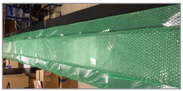
▲ Photo of completed LED ticker bars individually wrapped in protective bubble wrap and stored off the floor on a benchtop. It is important that these are handled with care when moving and avoid stacking anything.
