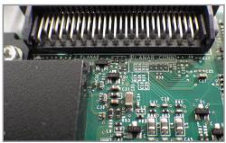
▲ Dell R520 network server circuitry after decontamination
