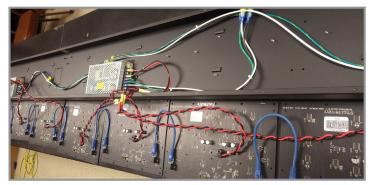
Ticker LED panel opened up for inspection and decontamination. Some water spotting identified and removed.
